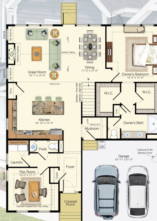
FIRST FLOOR Included Elevation A
