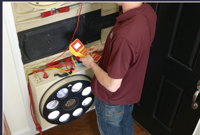
A Blower Door Test is performed on every Schell Brothers Home to obtain your home's HERS score.
